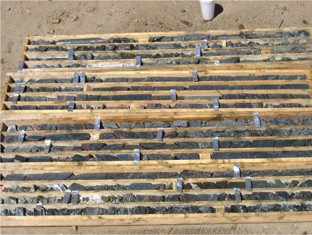
Figure 7. Drill Core (R04-5) from RAM deposit, Main Zone, Formation Capital Corporation's Idaho Cobalt Project.
