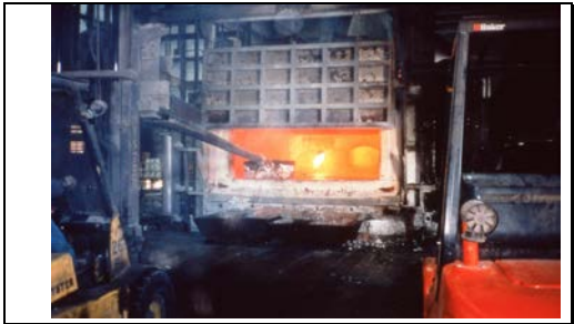
Imco, Inc, aluminum recycling, melting furnace
