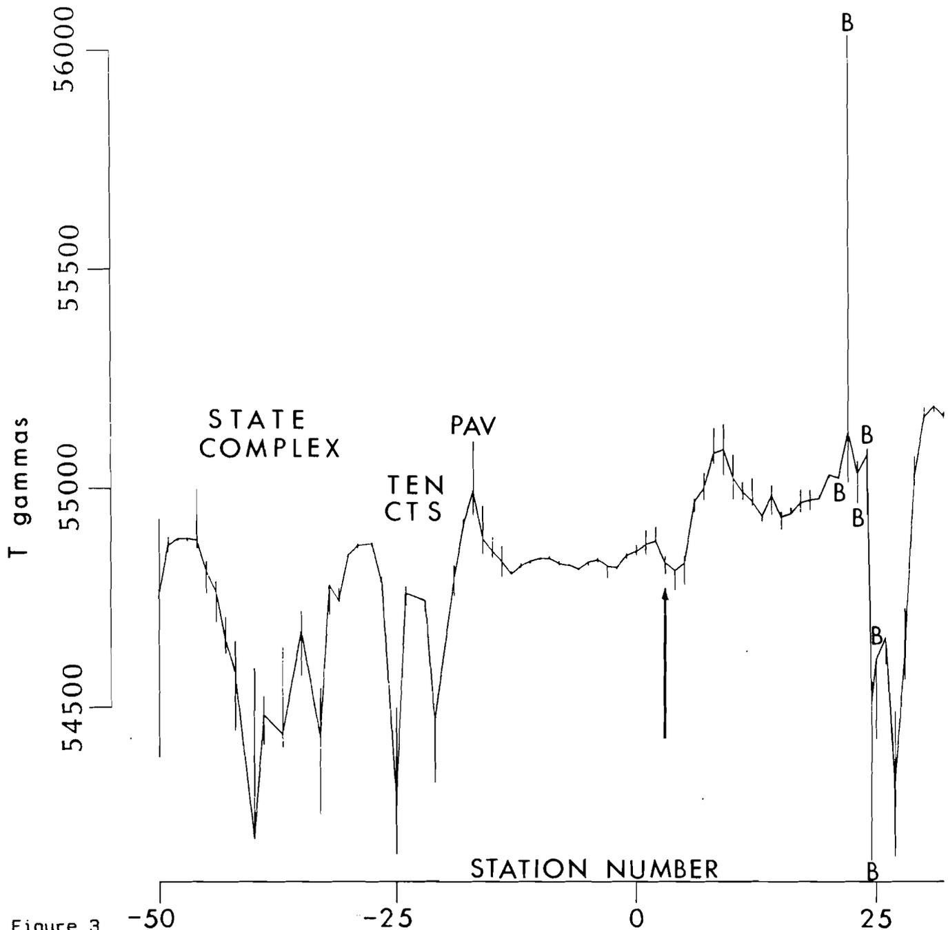
Figure 3 Detailed magnetic profile (western profile in Figure 2, top). Station spacing 10 paces = 28 feet approximately. Arrow indicates location of first break in slope. Symbols TEN CTS and PAV mean tennis courts and pavillion, respectively; B indicates station over basalt outcrop on upthrown side of fault. Vertical bars indicate minimum and maximum of: station reading, right lateral reading, left lateral reading; used to check horizontal gradient (see text).
