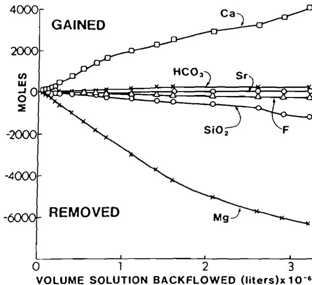
Figure 5. Gains and Losses during Test 2C, Raft River.
