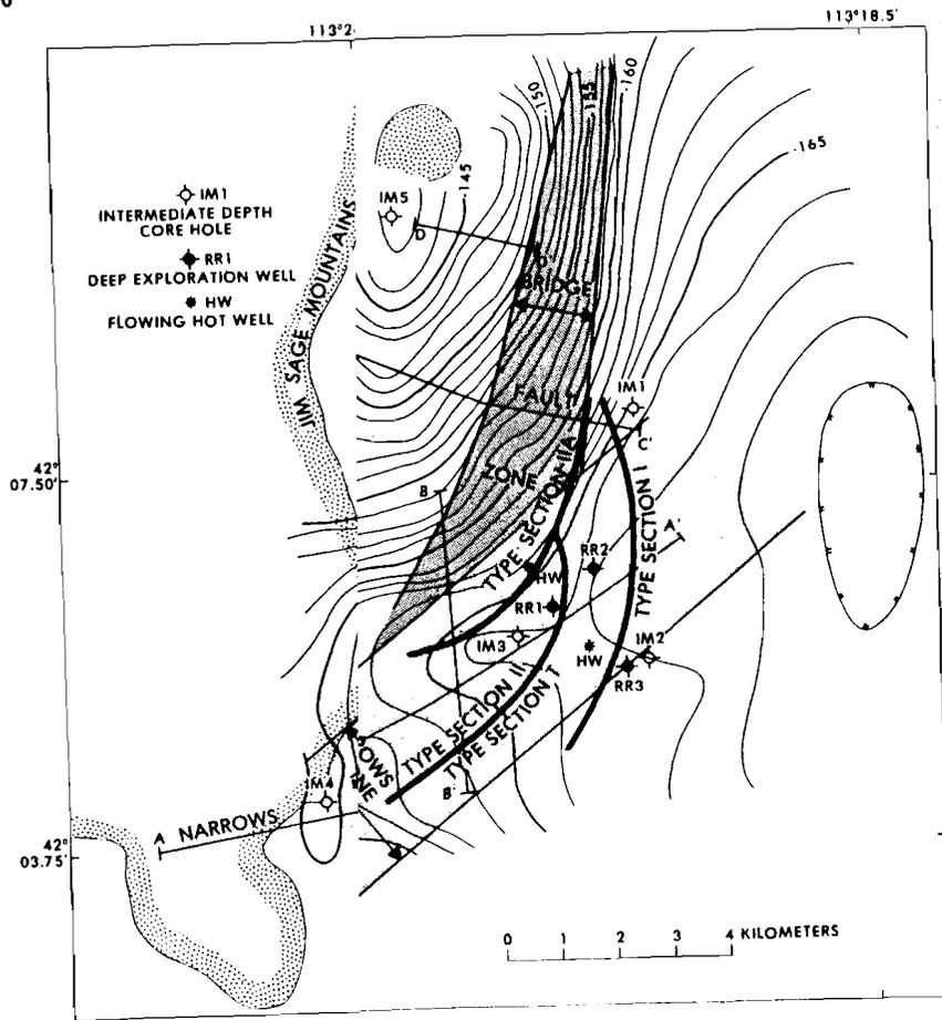
FIG. 3. Map showing locations of velocity sections A-A', B-B', C-C', and D-D', the boundaries of type sections I, T, II and IIA, the exploratory flowing hot wells, the Bridge fault zone, and the inferred Narrows zone and Bouguer gravity anomaly contours (Mabey et al, 1978).
