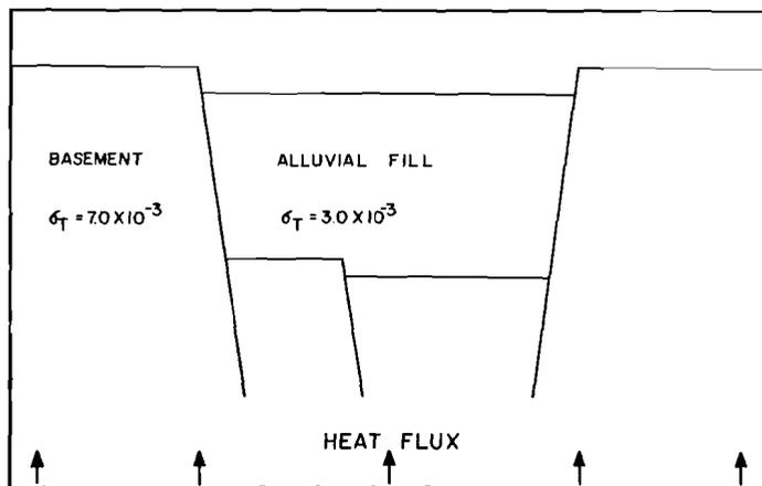
Fig. 12. Schematic diagram of the proposed geological model for the Boise, Cascade, and Raft River geothermal systems. Thermal conductivities ( $\sigma$ ) of  $3.0 \times 10^{-3}$  and  $7.0 \times 10^{-3}$  cal/cm s  $^{\circ}$ C were used for the sediments and basement rock, respectively, to calculate the temperatures at the base of the sedimentary section.
