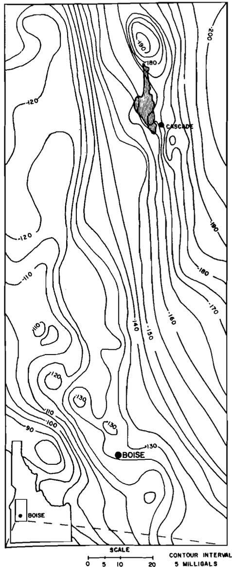
Fig. 5 Regional gravity map of a portion of west central Idaho showing the apparent lack of shallow intrusives [Mabey et al. 1974].
