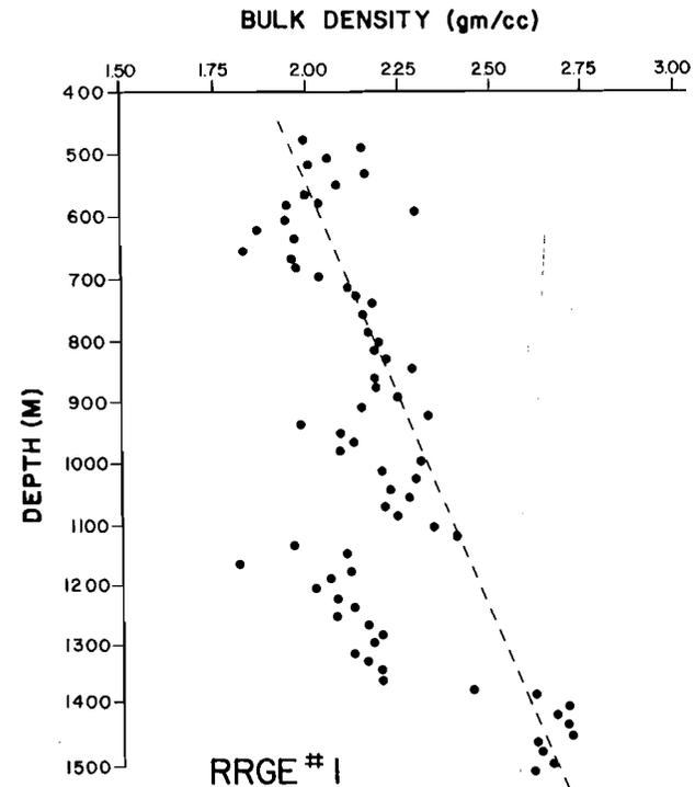
Fig. 11. Plot of bulk density from density log versus depth for RRGE #1. The general trend is that density increases with depth in a sedimentary sequence because of increasing compaction and decrease of porosity. The graph then shows a decrease in porosity with depth until the productive zone (1150 to 1370 m) is encountered [Applegate et al., 1976].
