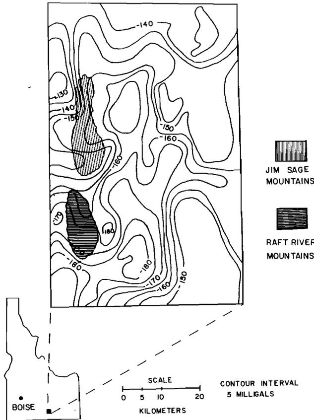
Fig. 10. Gravity map of the Raft River Valley. The Narrows structure separates the Jim Sage Mountains from the Raft River Mountains. The Bridge fault is along the eastern flank of the Jim Sage Mountains. Gravity data is from Mabey et al. [1974].
