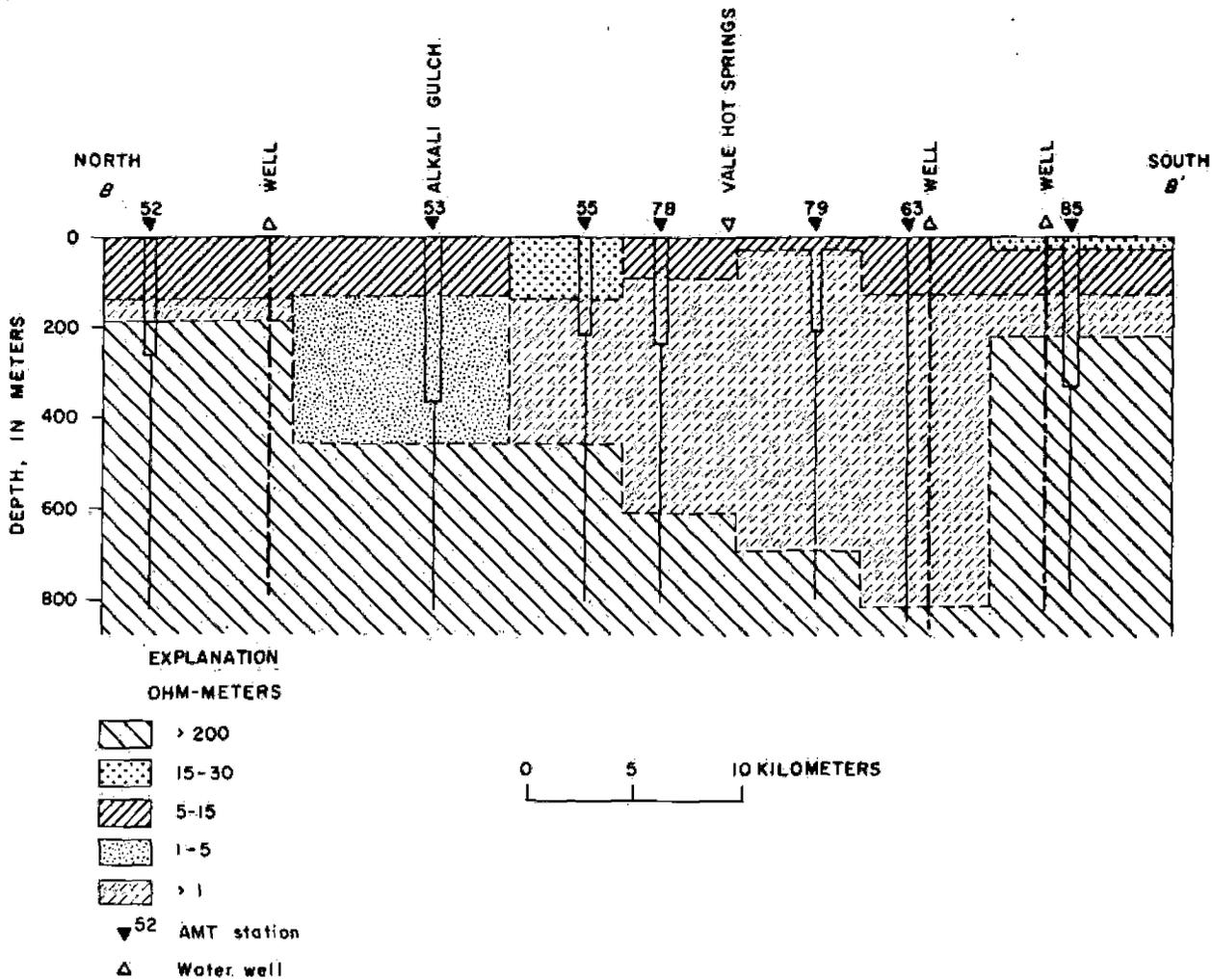
FIG. 5. Electrical cross-section.
