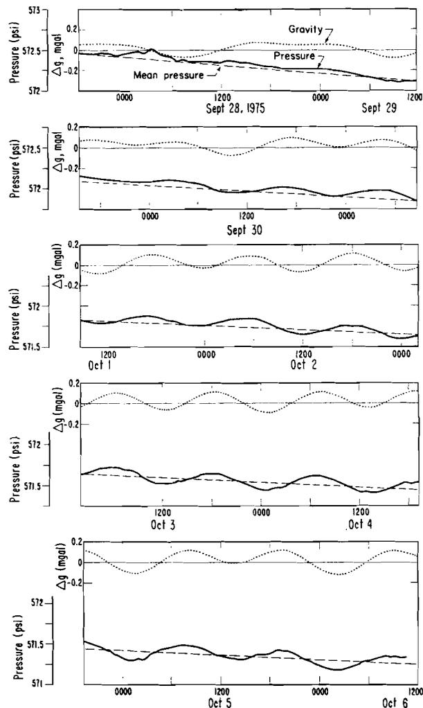
Fig. 3—Correlation between variation in the earth's gravitational field and water pressure in Well RRGE 1 during the interference test.
