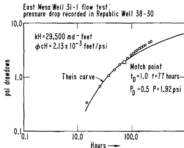
Fig. 10—Interference test, Well RG 38-30: Log-log plot of time vs drawdown.
