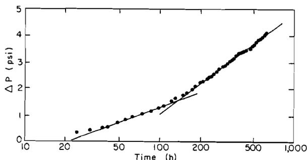
Fig. 7—Interference test, Well RRGE 1: Semilog plot of time vs drawdown.
