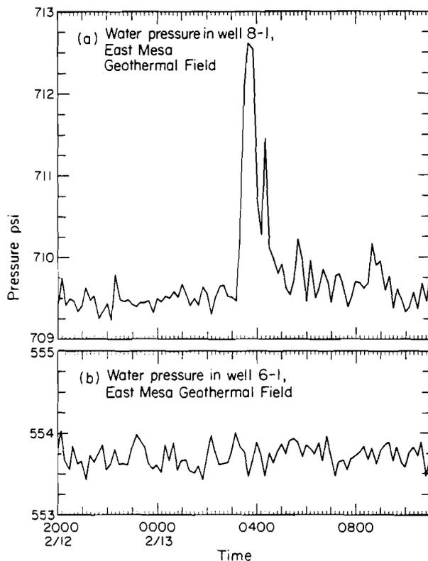
Fig. 5—Comparison of water pressure fluctuations in Well EM 8-1 with Well EM 6-1 recorded before the start of the first interference test.
