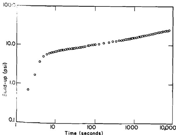
Fig. 8—Short-term production test, Well RRGE 2: Log-log plot of buildup vs time.
