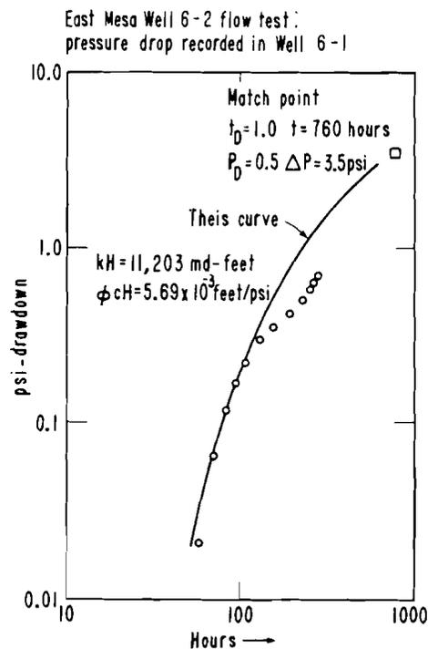
Fig. 9—Interference test, Well 6-1: Log-log plot of time vs drawdown.
