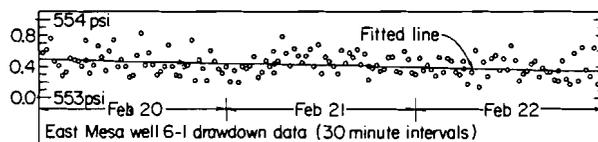
Fig. 4—Comparison of the pressure data recorded in Well EM 6-1 during the first interference test with the fitted line used for analysis.
