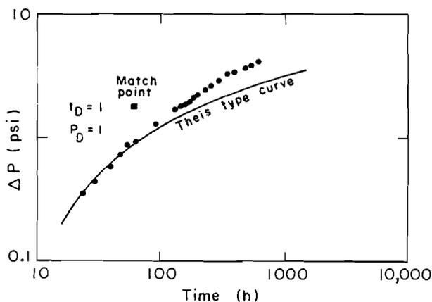
Fig. 6—Interference test, Well RRGE 1: Log-log plot of time vs drawdown.
