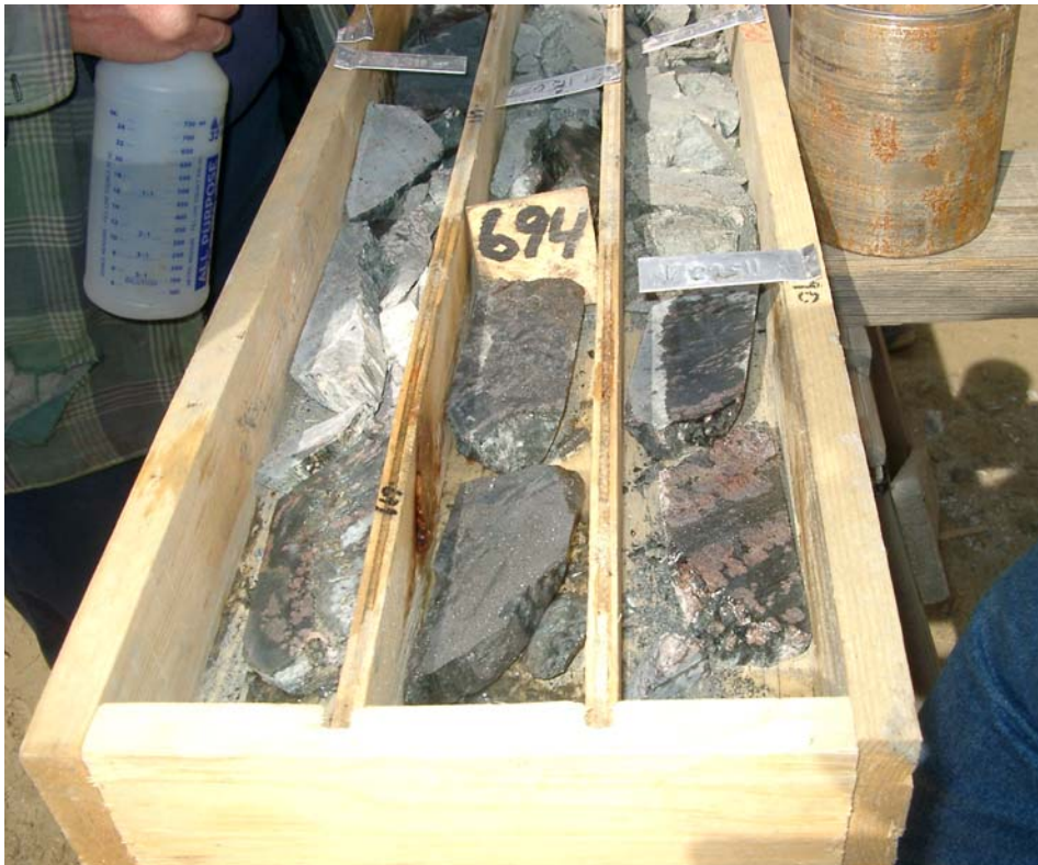
Figure 8: Formation Capital Corporation's Idaho Cobalt Project. Drill core from R05-03, 694' with massive pinkish cobaltite intercept in garnet-biotite schist.
