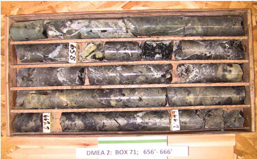
Figure 8. Massive sulfide and skarn from Thunder Mountain Gold's South Mountain property, Owyhee County, Idaho.
