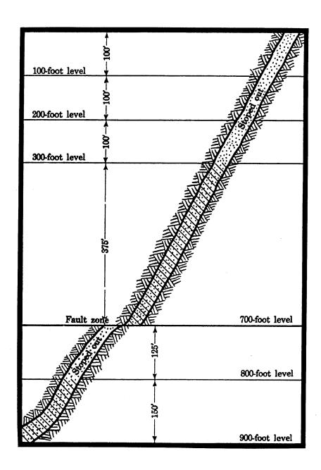
Figure 7. Cross section of the Harmony Mine from the 900-foot level to the surface (Figure 1 from Gardner, 1930a).
