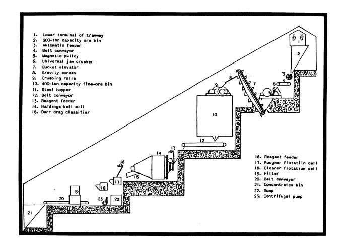
Figure 5. Side view of the Harmony mill, showing the position of the machines (Figure 2 from Gardner, 1930b).
