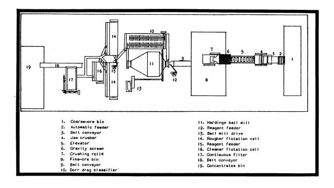
Figure 6. Plan of the Harmony mill (Figure 3 from Gardner, 1930b).
