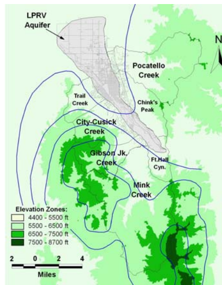
Figure 3 - Hypsography of the LPRV compared to mean annual precipitation (isohyets taken from Figure 2). Areas of principal snowpack accumulation occur at the highest elevations (darkest shading), which coincide with areas of highest annual precipitation.
